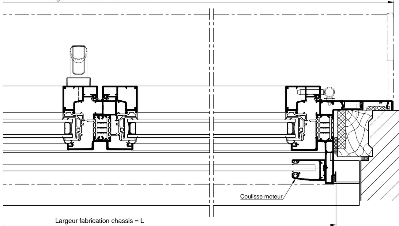
**AVEC COUVRE-JOINT INTERIEUR AVEC GRAND CLIP ( CAS COMMANDE MANUELLE OU DE SECOURS )**
